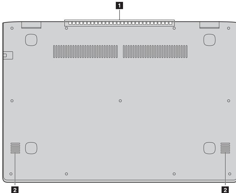
**1 Ventilation slots** Dissipate internal heat.
