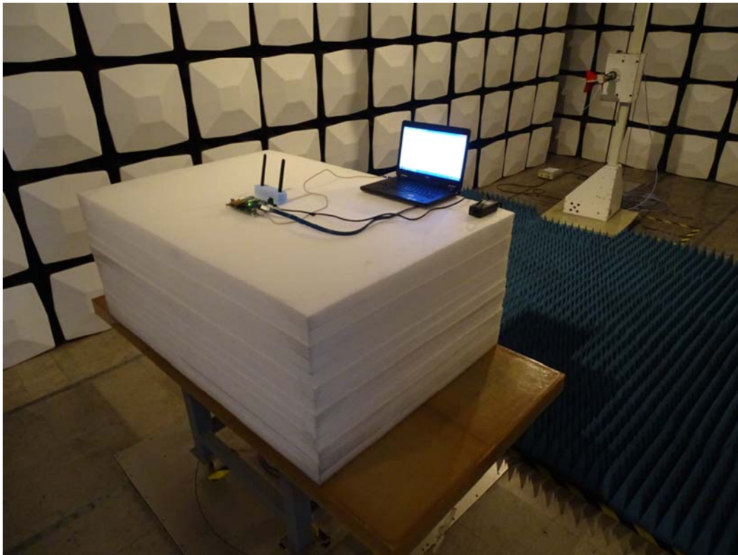
Front View of Radiated Test (Horn)
