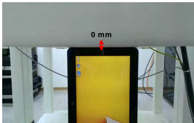
Fig.5 EUT left side to flat phantom
