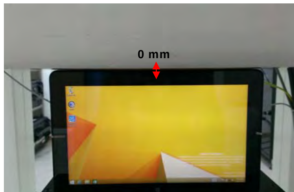
Fig.4 EUT top side to flat phantom
