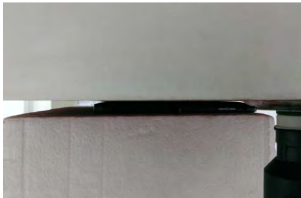
Fig.3 EUT lap-held mode to flat phantom
