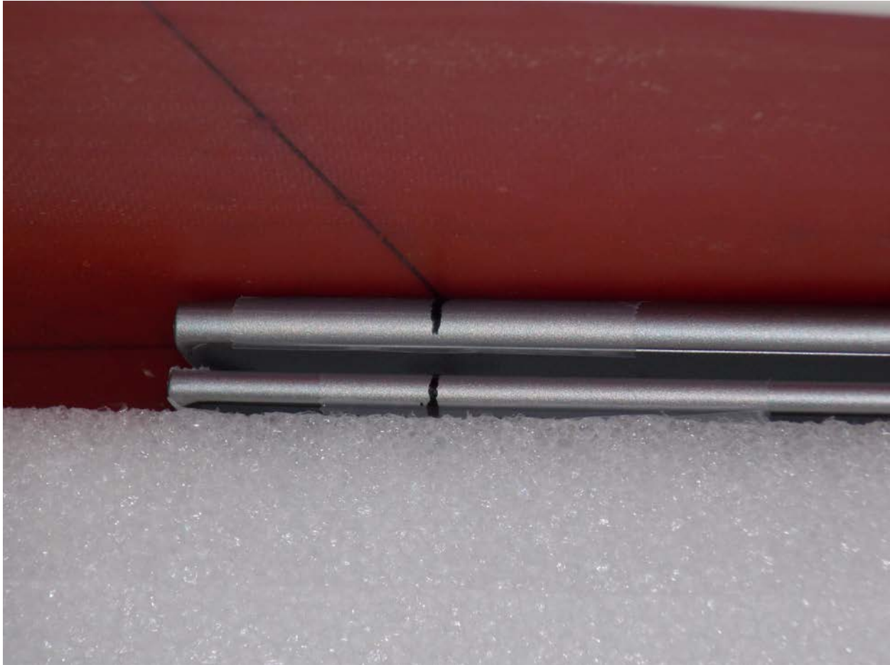
Test Position Tablet Mode Back 0 mm Gap
