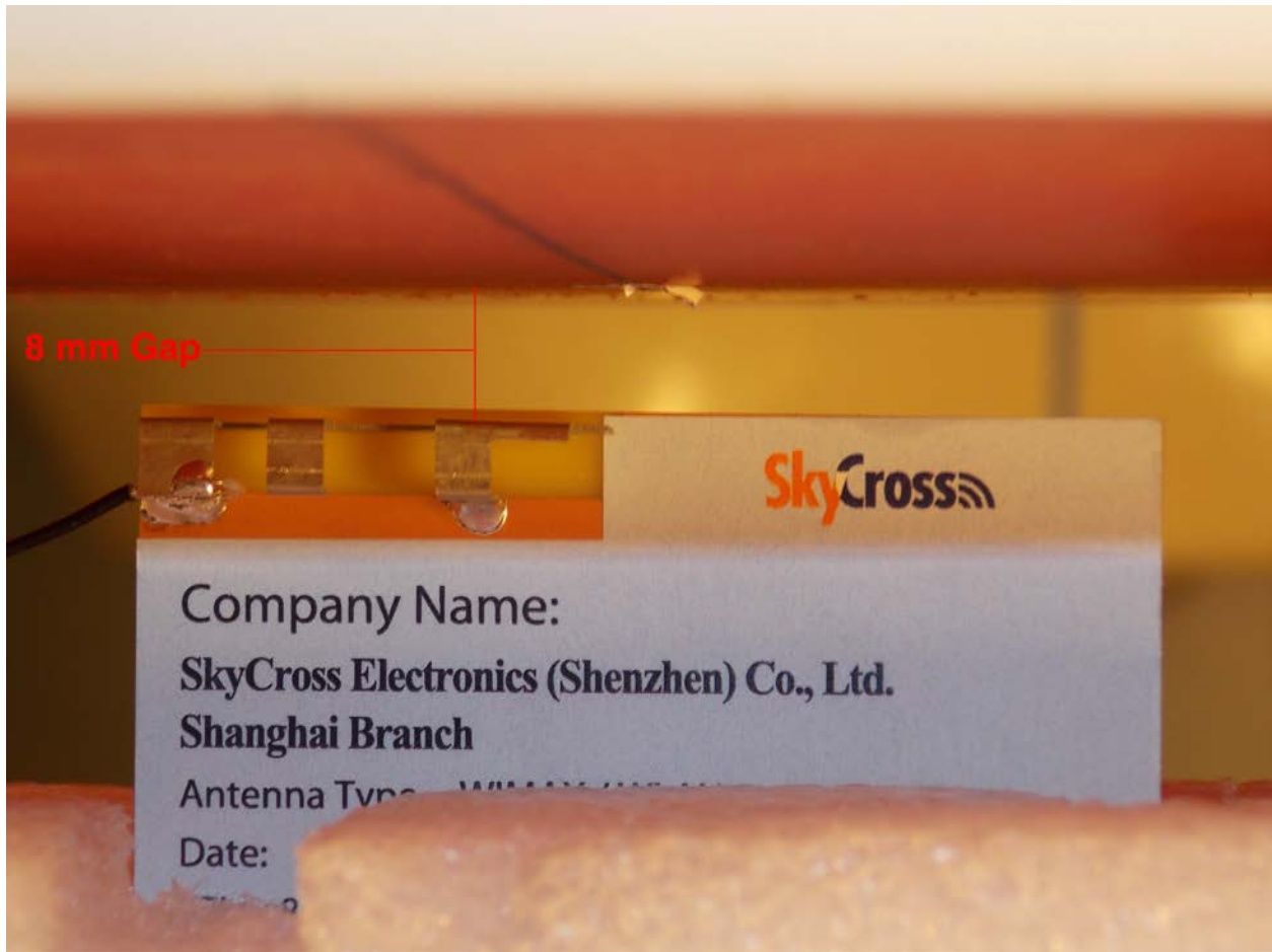
Test Position Side D 8 mm Gap
