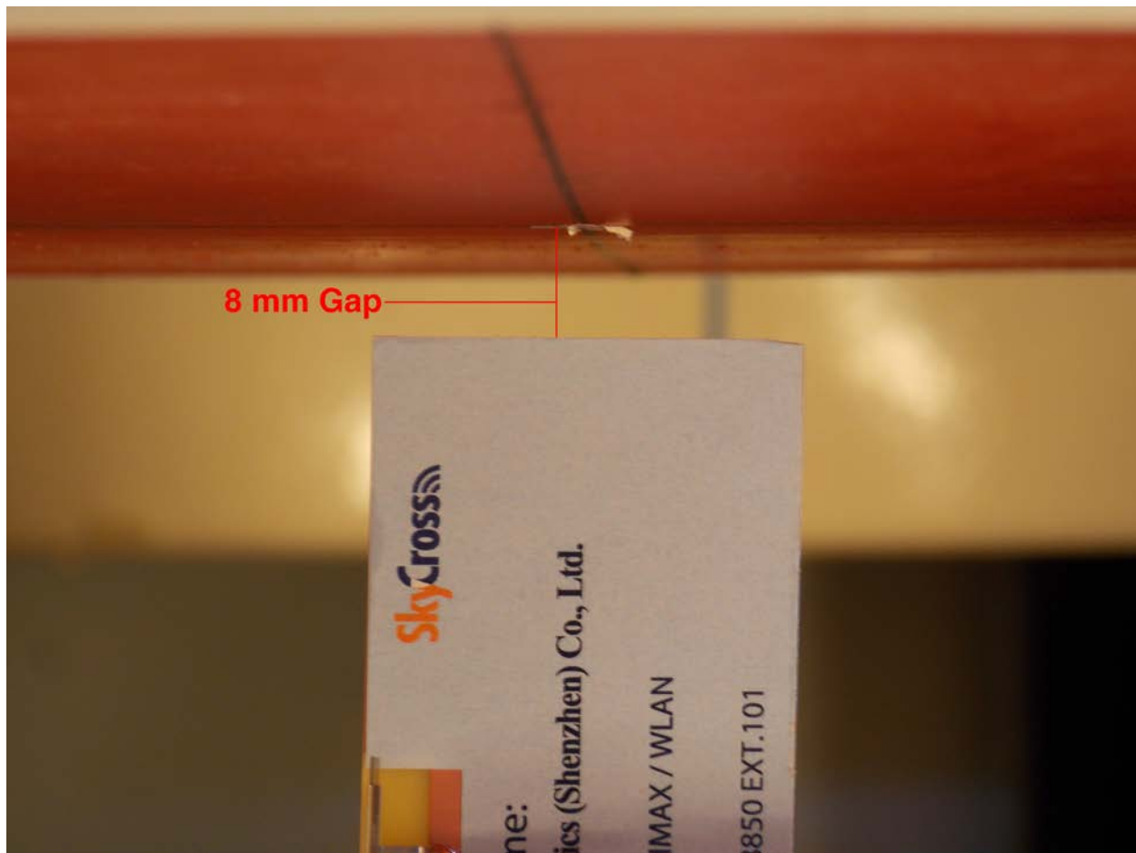
Test Position Side E 8 mm Gap
