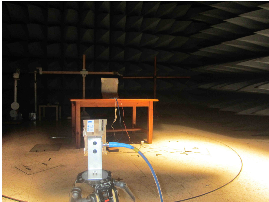
Fig. 6. Test set-up for radiated measurements above 18GHz to 26GHz
