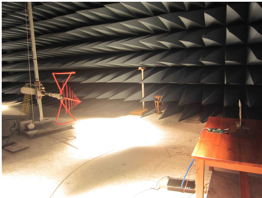
Fig. 4. Test set-up for radiated measurements above 30MHz to 1GHz
