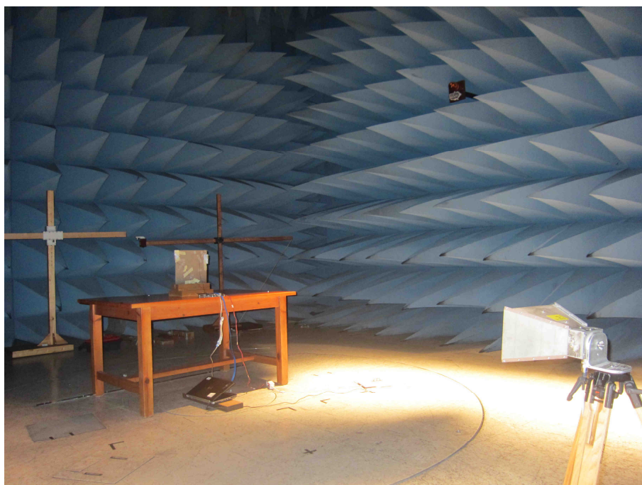
Fig. 5. Test set-up for radiated measurements above 1GHz to 18GHz
