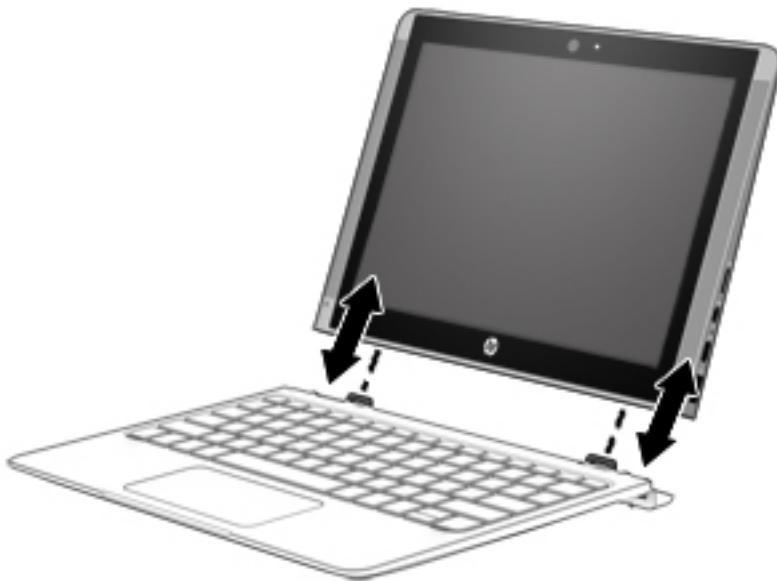
**CAUTION:** If your keyboard contains a hard drive, disconnect the hard drive before you remove the keyboard. If the keyboard is not disconnected before it is removed, the hard drive could be damaged, and data files might be corrupted.
