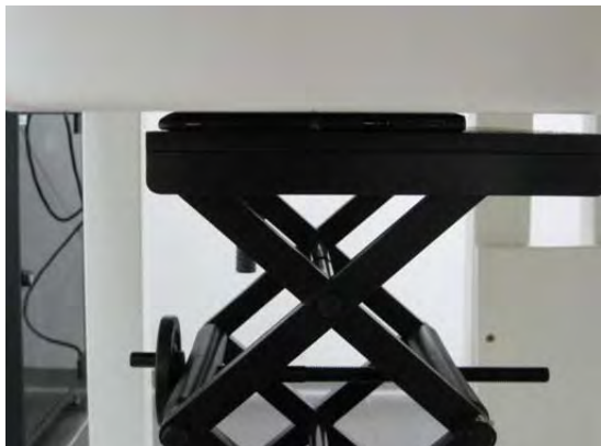
Fig.3 EUT lap-held mode to flat phantom
