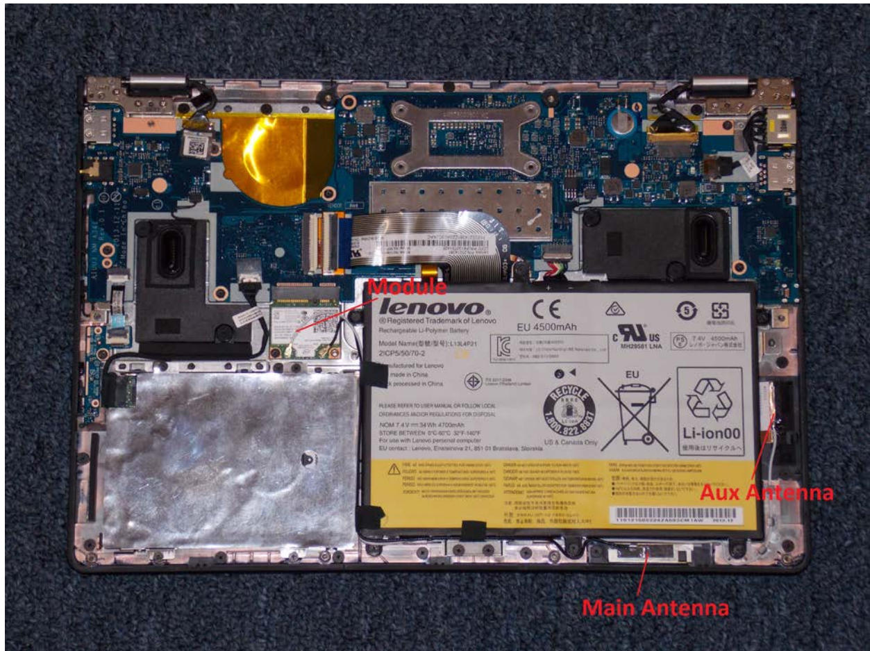
Module and Antenna Locations
