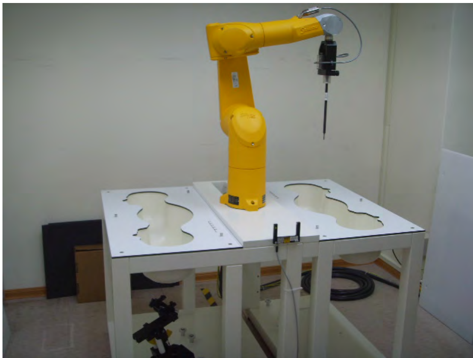
Fig.1 Photograph of the SAR measurement system
