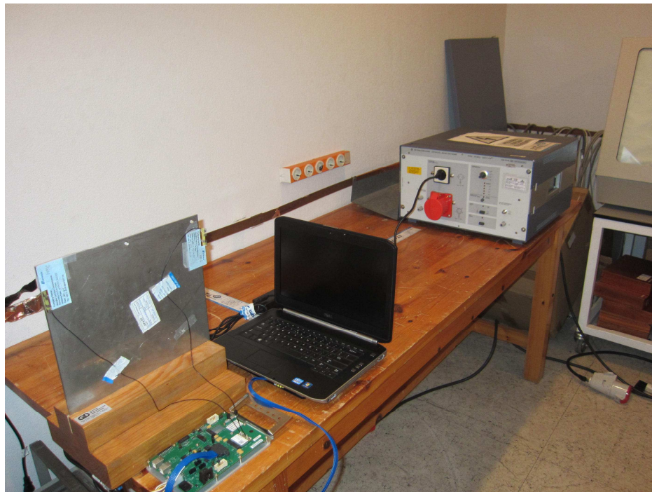
Fig. 7. Test set-up for conducted measurements
