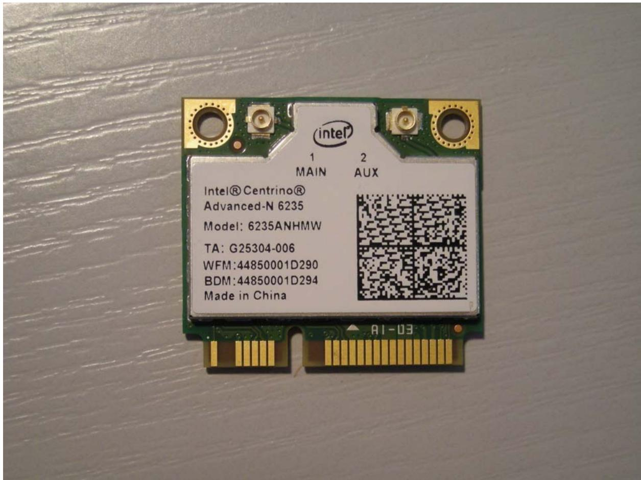
Photos shows label placement on half-mini card
