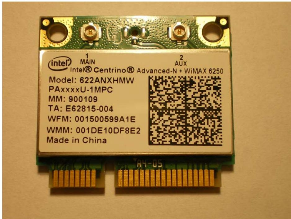
Photo showing label placement on half-mini card.
