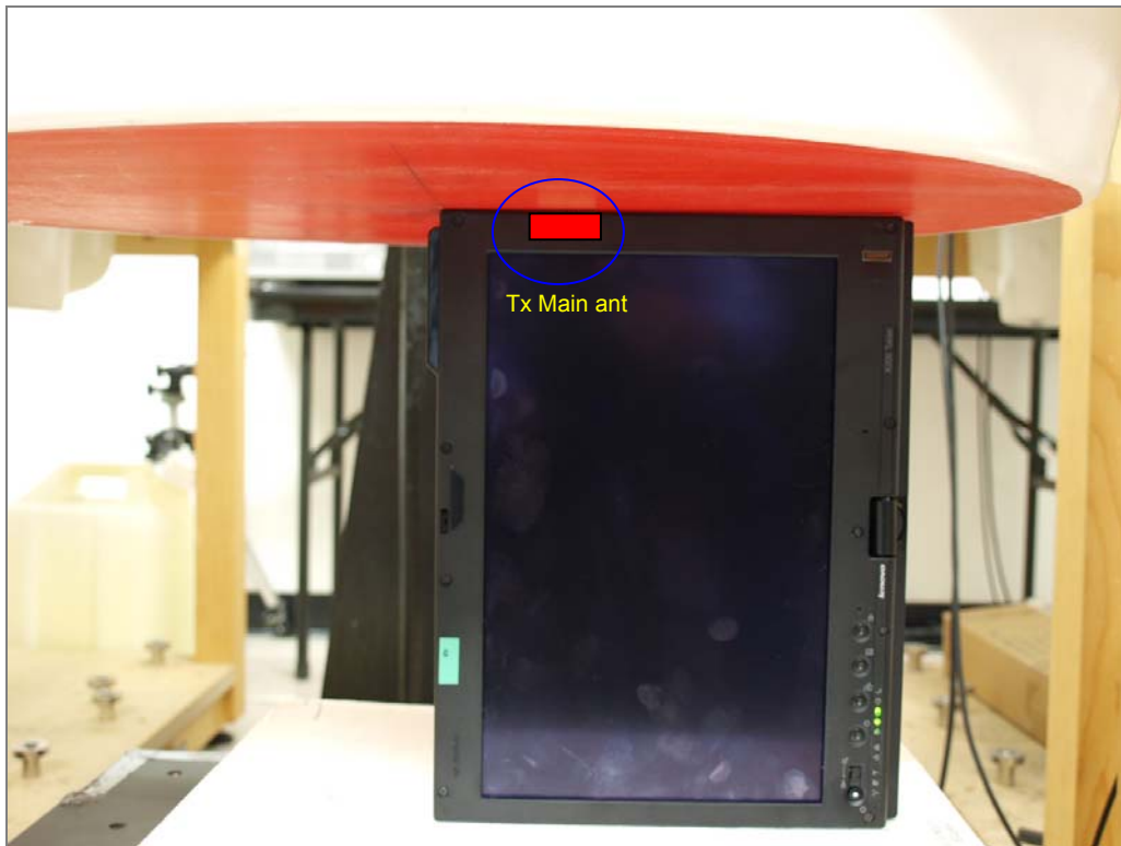
Separation distance between Tx antenna-to-flat phantom
