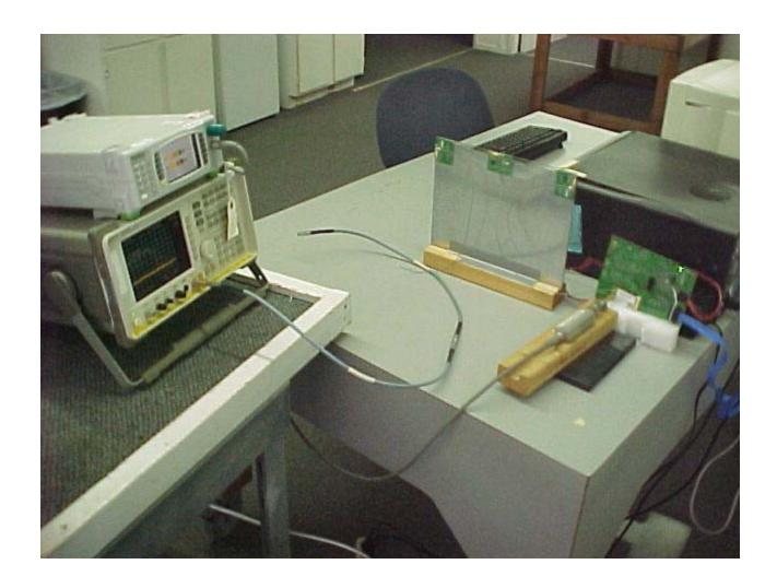
Maximum Peak Output Power Measurement Setup
