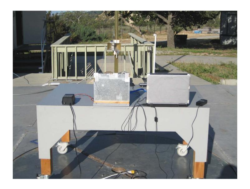
Radiated Emissions Measurement (Rear View) WiFi Setup
