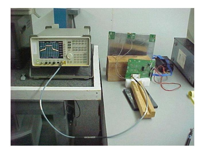
Conducted Emissions at Antenna Terminal Setup
