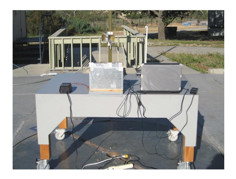
Radiated Emissions Measurement (Rear View) WiMax Setup
