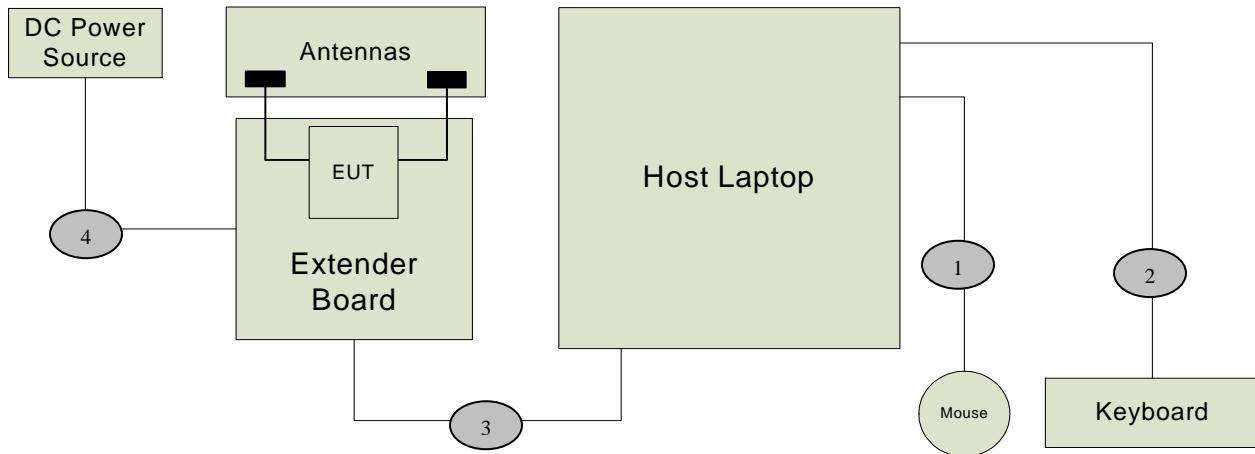
Remotely Located from EUT setup
