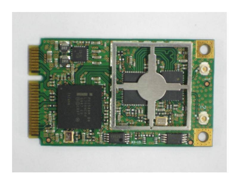
Top View "Shielding removed"
