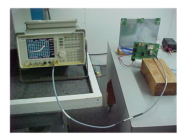
Conducted Emissions at Antenna Terminal Setup
