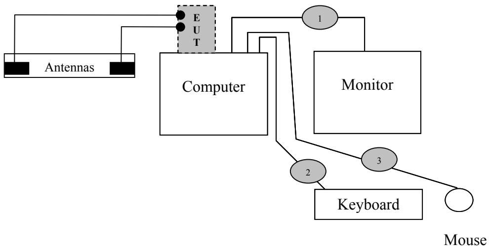
Cable 1: This is a 6-foot braid and foil shielded round cable connecting the host computer with the monitor. It has metallic DB-15 type connector at the computer end and is hardwired to the monitor. The cable is bundled to a length of one meter and the shield of the cable is grounded to the chassis of both devices via the connector shells.
