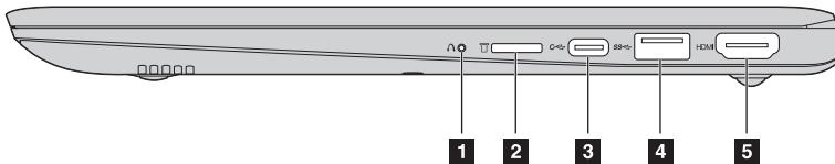
**1 Novo button** When the computer is off, press this button to start the System Recovery or the BIOS setup utility, or to enter the boot menu.
