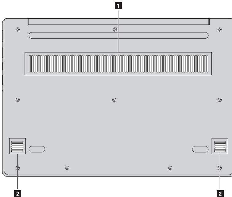
**1 Ventilation slots** Dissipate internal heat.
