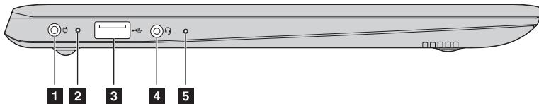
**1 AC power adapter jack** Connects to the AC power adapter.
