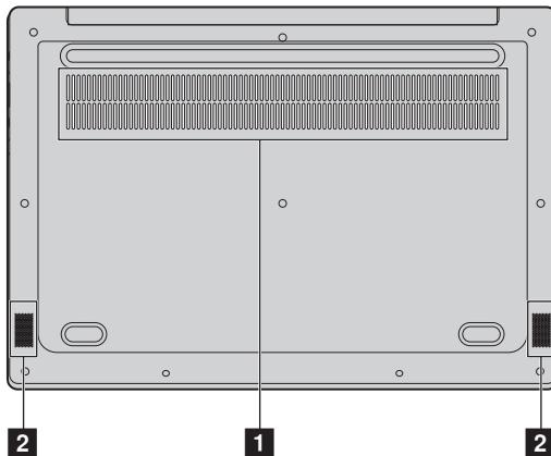
**1** **Ventilation slots** Dissipate internal heat.
