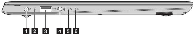
**1 AC power adapter jack** Connects to the AC power adapter.
