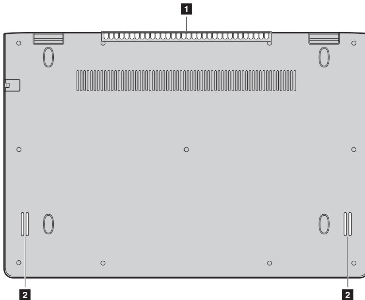
**1 Ventilation slots** Dissipate internal heat.
