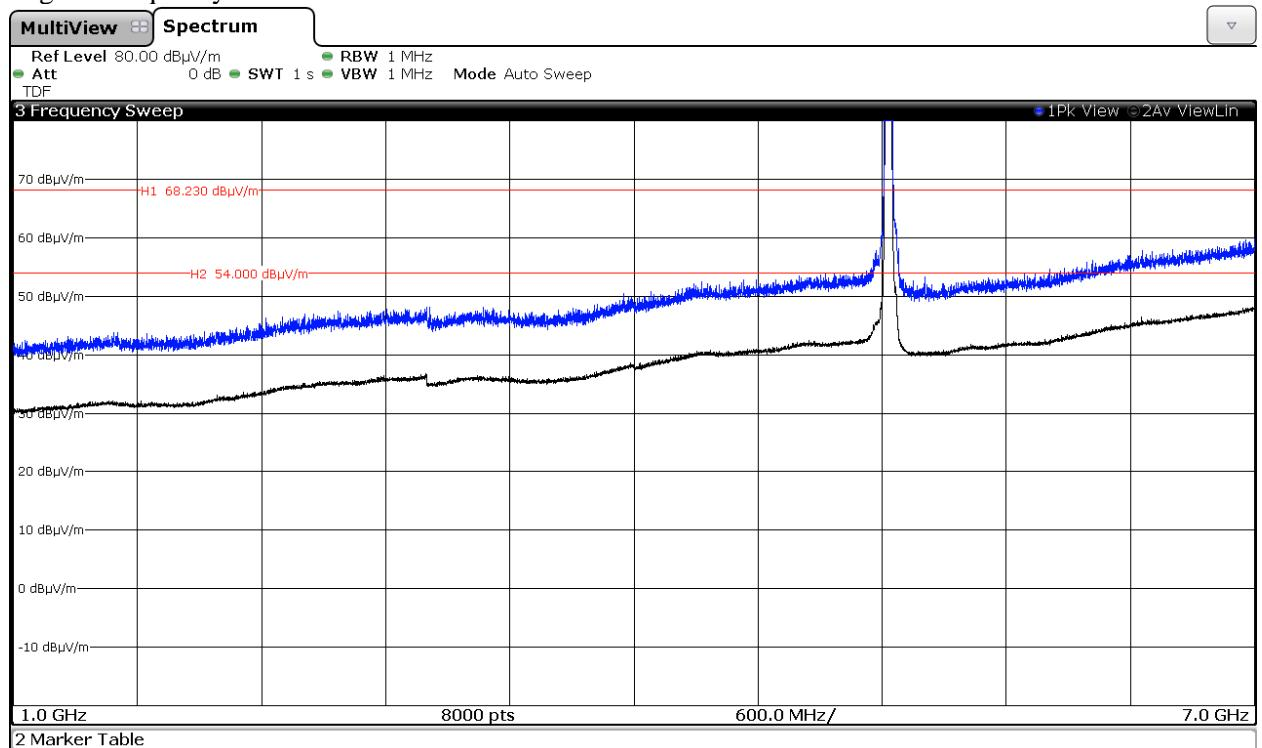
The peak above the limit is the carrier frequency. This plot is valid for Chain A, Chain B, Chain A+B.
