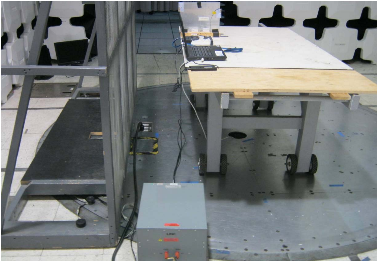
Test Configuration Photograph #2 (Conducted Emissions - Power Port)
