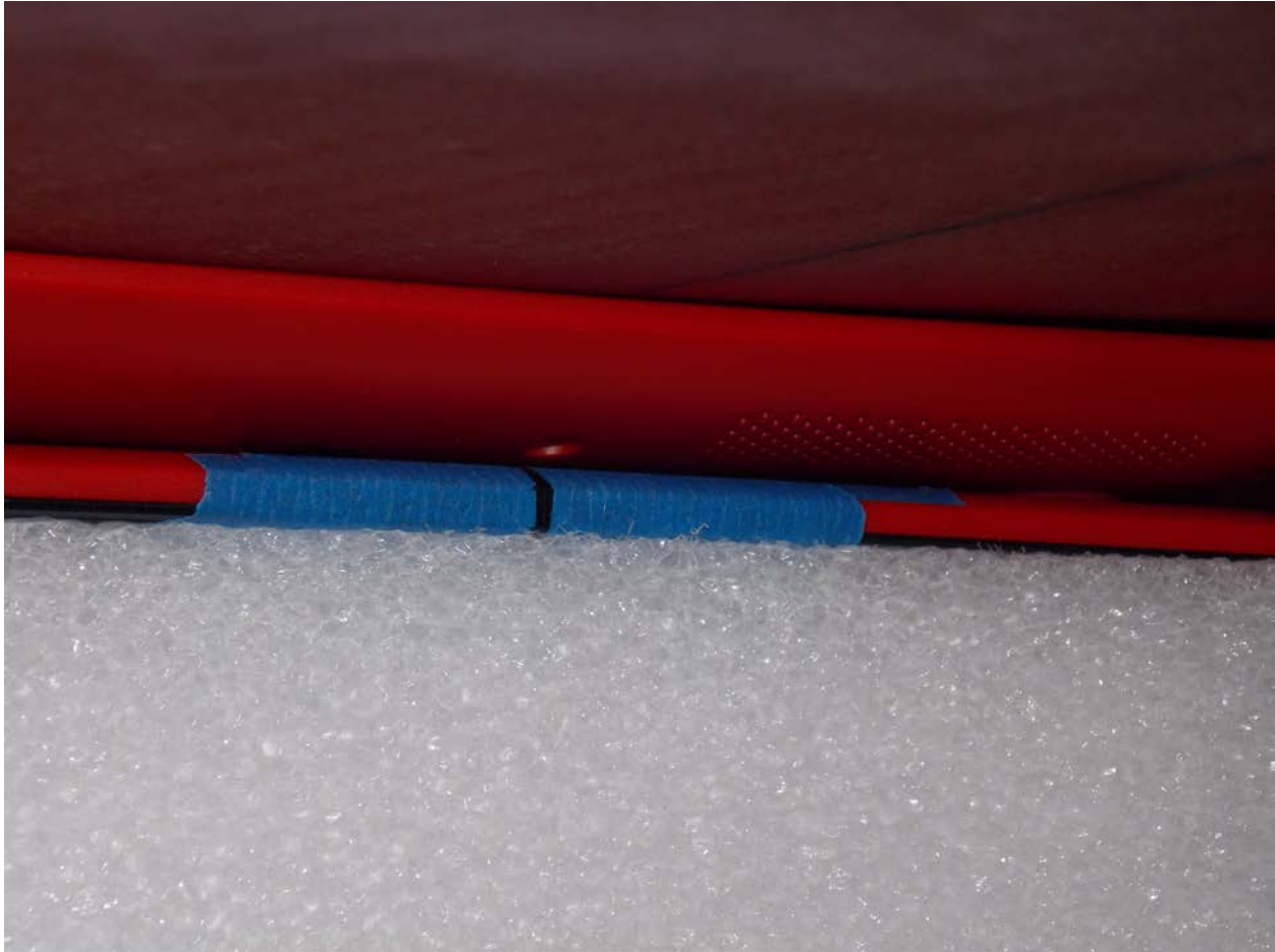
Test Position Tablet Back 0 mm Gap
