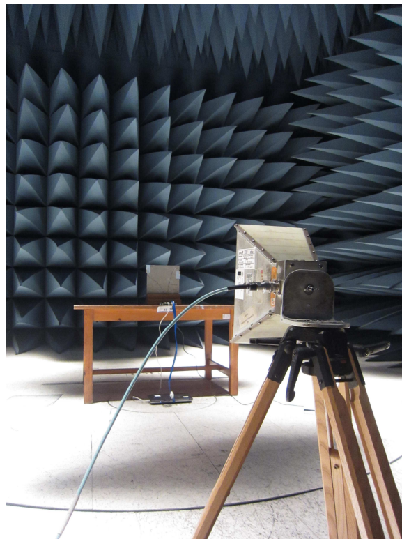
Fig. 5. Test set-up for radiated measurements above 1GHz to 18GHz
