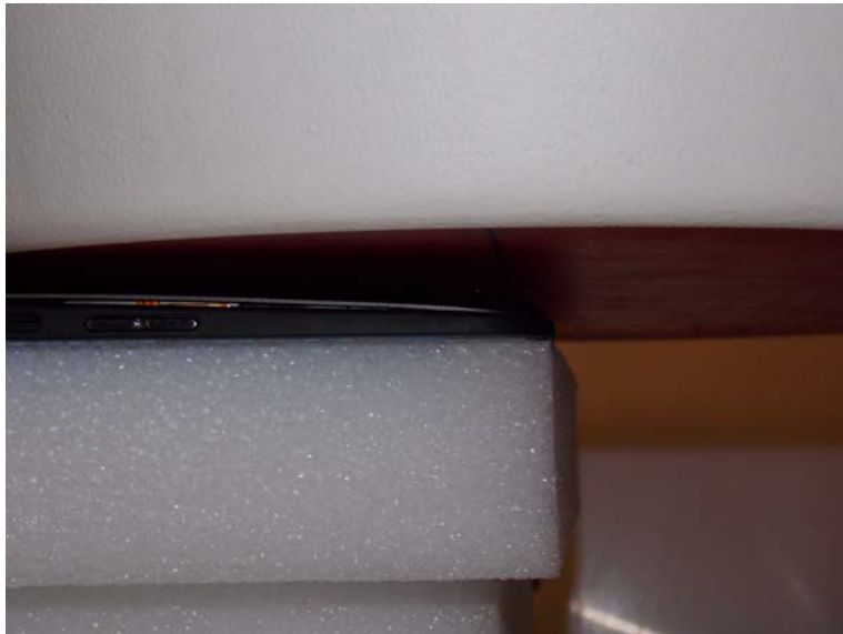
Test Position Back Both Antennas 0 mm Gap
