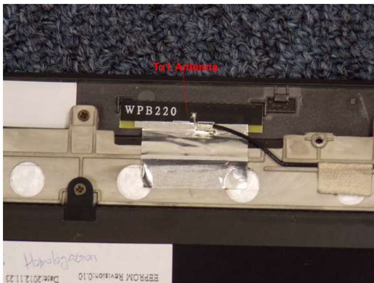
Close up of Tx1 Antenna
