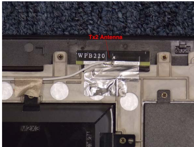
Close up of Tx2 Antenna
