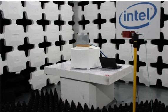
A photograph showing a test setup in a chamber with a white and black cross-hatched absorber wall. A white rectangular device is mounted on a white rectangular stand. A yellow vertical rod is positioned behind the device. A blue light is visible on the horn antenna. A black metal frame is visible on the right side of the image. |
