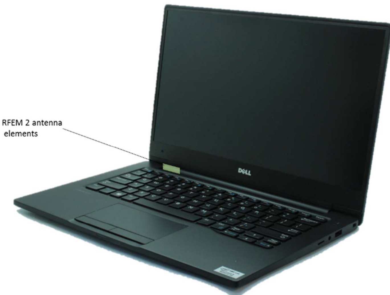
Figure 6 – Active antenna inside the platform
