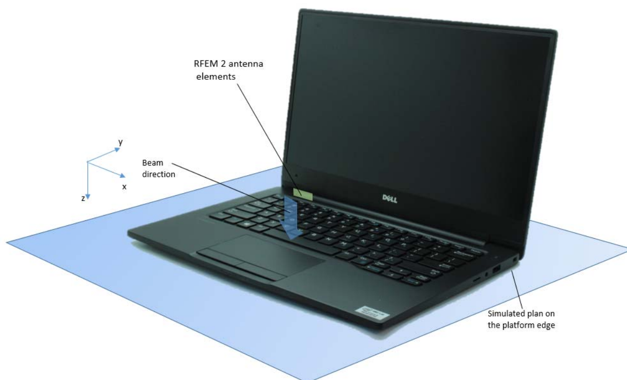
Figure 3 – Search Plane is the x-y plane (i.e. the blue plane as illustrated in this picture)
