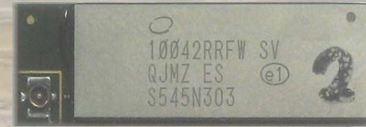
The RFEM2 is populated and the shield is molded onto the board at the same time. When the shield is removed the board is destroyed so there are no front without shield photos for the RFEM2. Photo revised to show 18260NG module.
