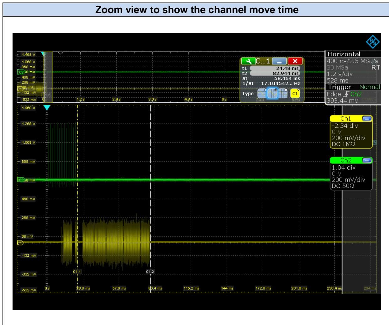
On the screenshot above, the cursors are placed between the latest radar signal and the latest data packet transmitted by the EUT to the master device. The time delta value show the channel move time, here the value is 58.46 ms.
