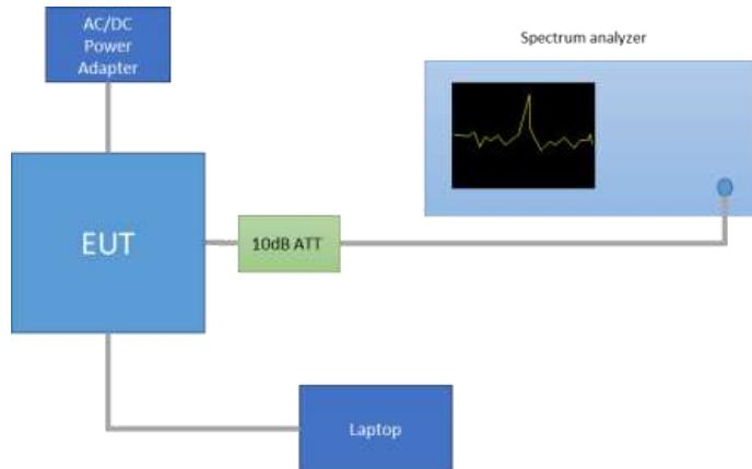
Note: these  $PSD_{Peak}$  values are shown just as a reference for the compliance of the Out-of-band Measurements. Thus the RBW used for these measurements was 100 kHz.
