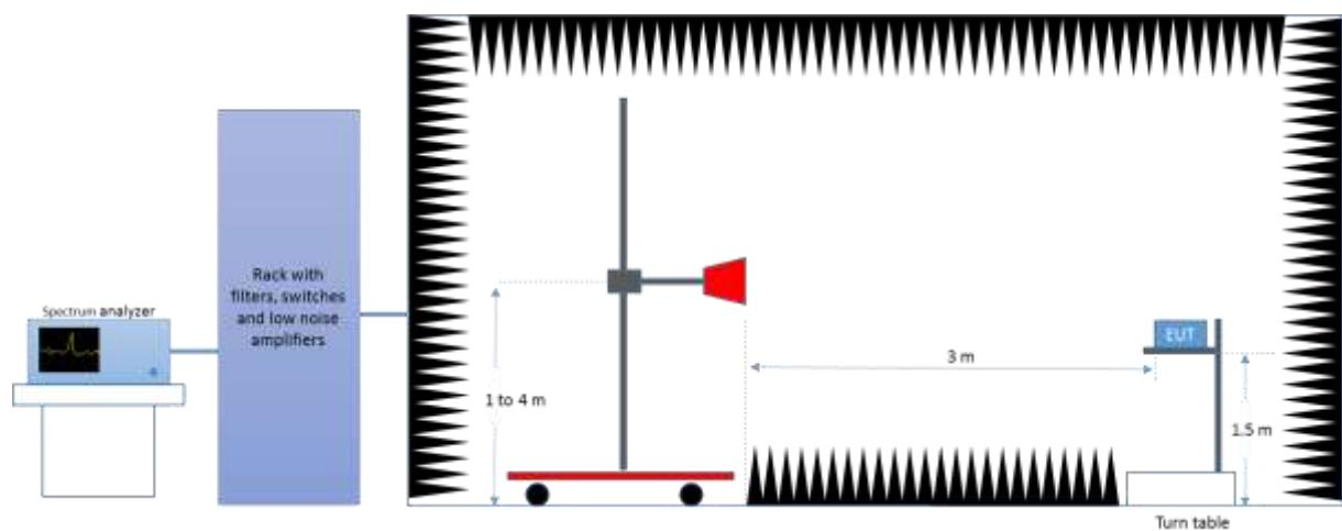
*Radiated Setup > 18GHz*
