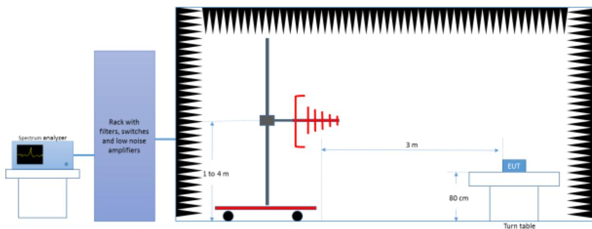
*Radiated Setup 1GHz - 18GHz*
