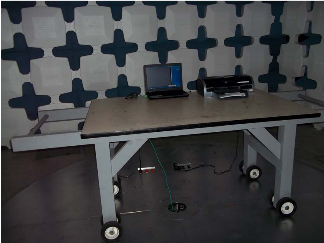
Radiated Emissions Test Configuration Photograph
