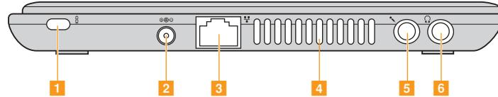
**1 Kensington slot** Attach a security lock (not supplied) here.
