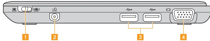
**1 Integrated wireless device switch** Use this switch to turn on/off the wireless radio of all wireless devices on your computer.
