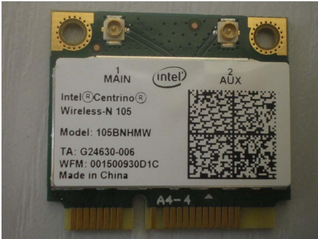
Photos shows label placement on half-mini card
