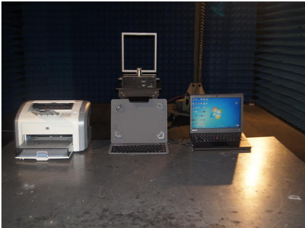
Photograph 6: Set-up for Radiated Emissions, 9 KHz-30MHz
