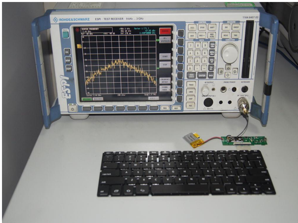
Photograph 8: Set-up for radio spectrum test
