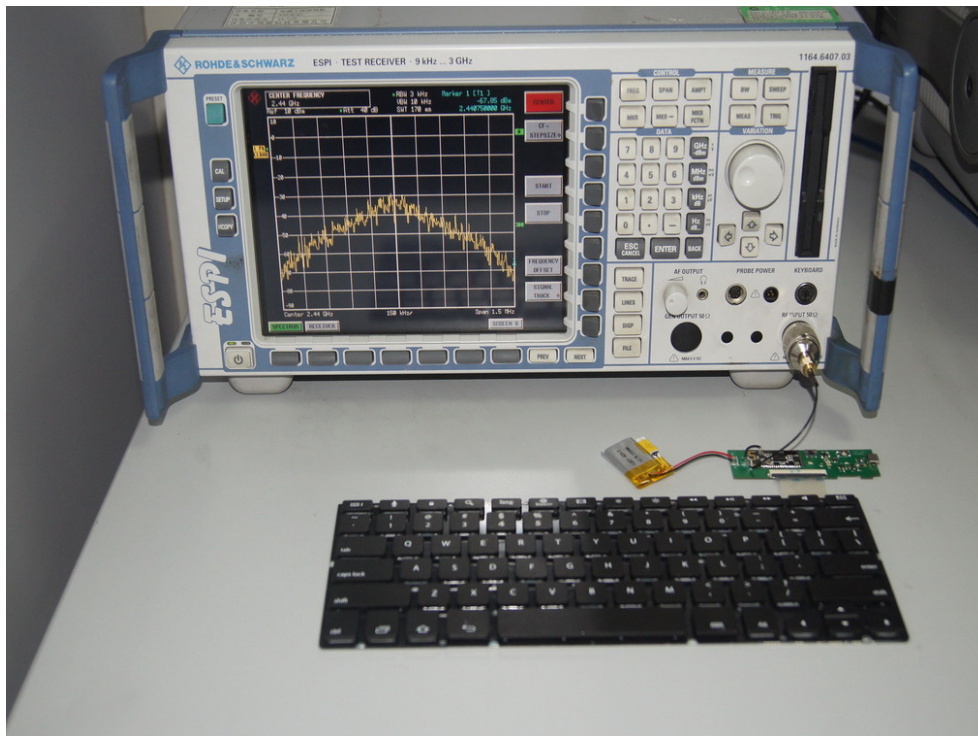
Photograph 8: Set-up for radio spectrum test
