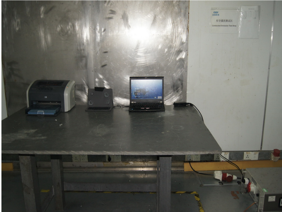
Photograph 6: Set-up for Radiated Emissions, 9 KHz-30MHz
