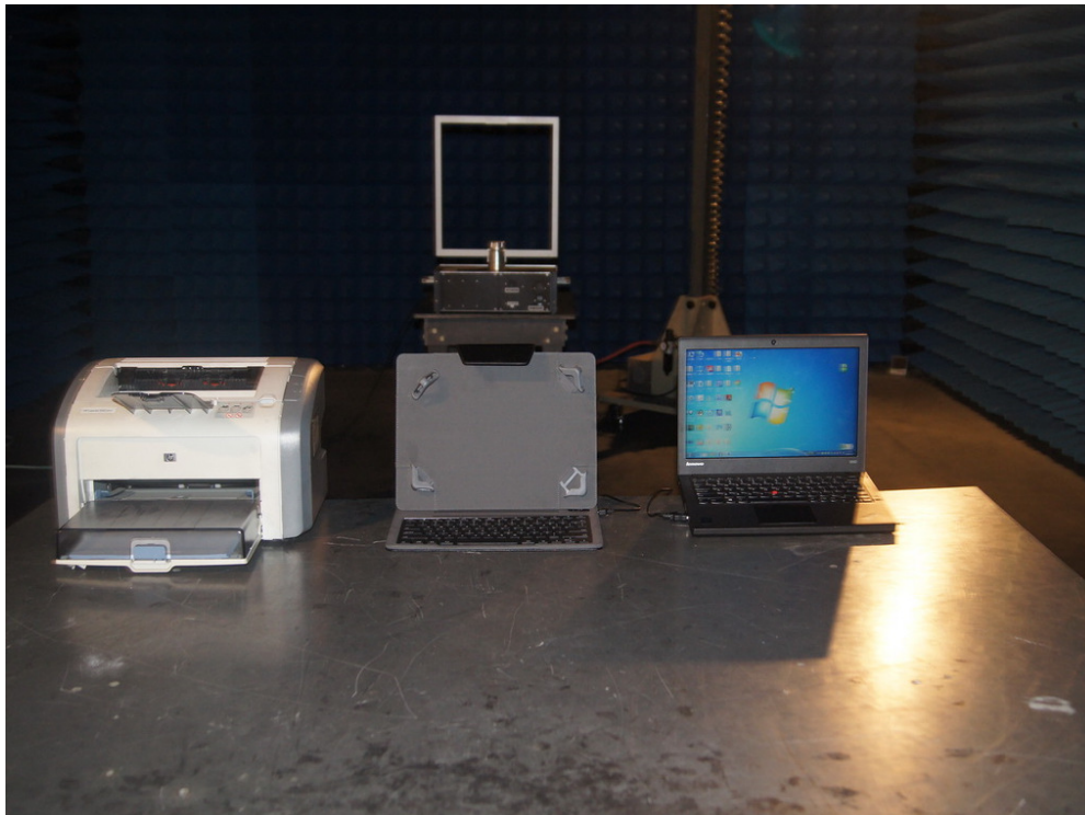
Photograph 6: Set-up for Radiated Emissions, 9 KHz-30MHz
