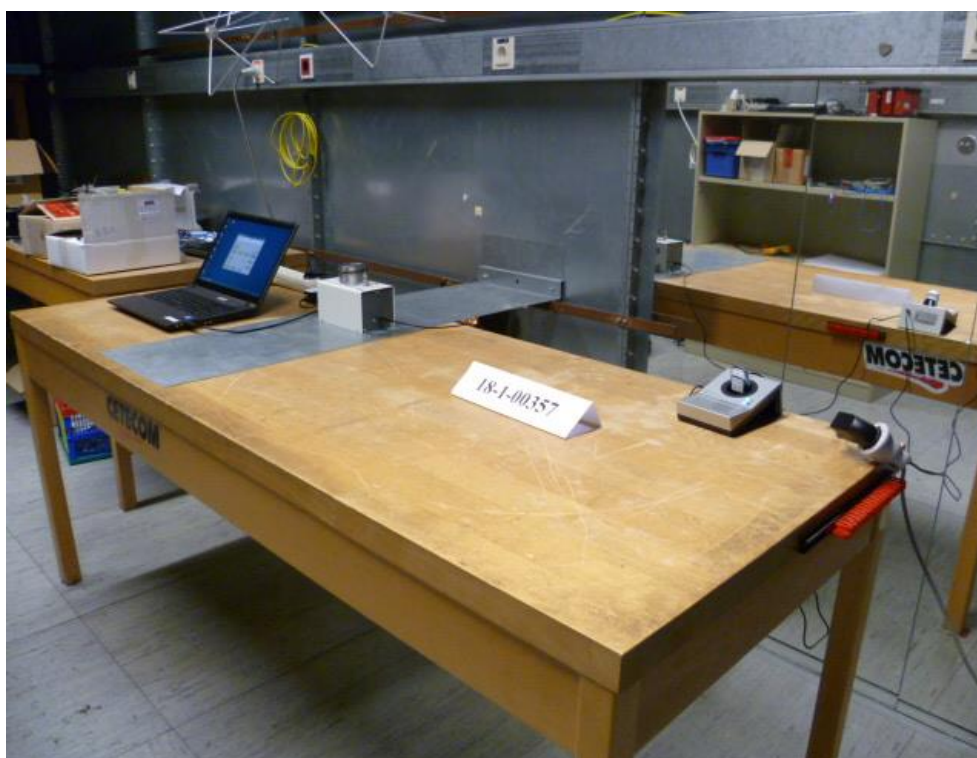
Photograph 2: EUT_Setup for AC power-line conducted emission measurements
