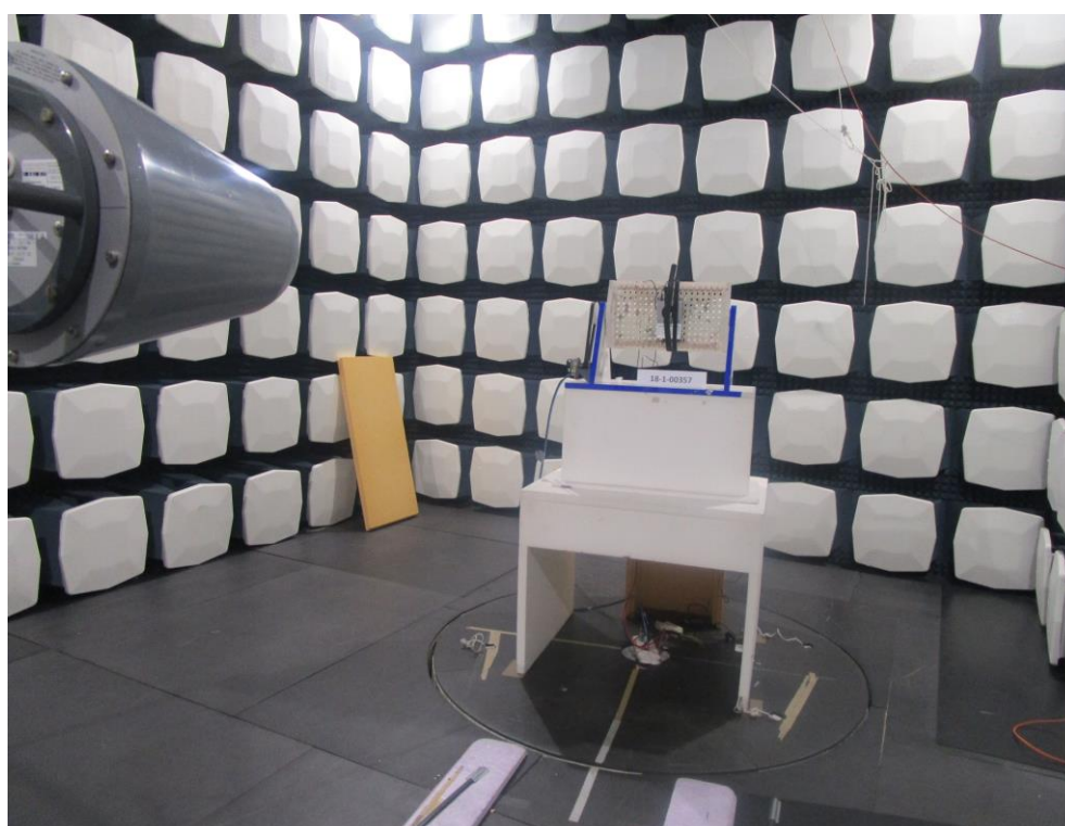
Photograph 6: EUT_Setup_overall view in the Full-anechoic chamber
