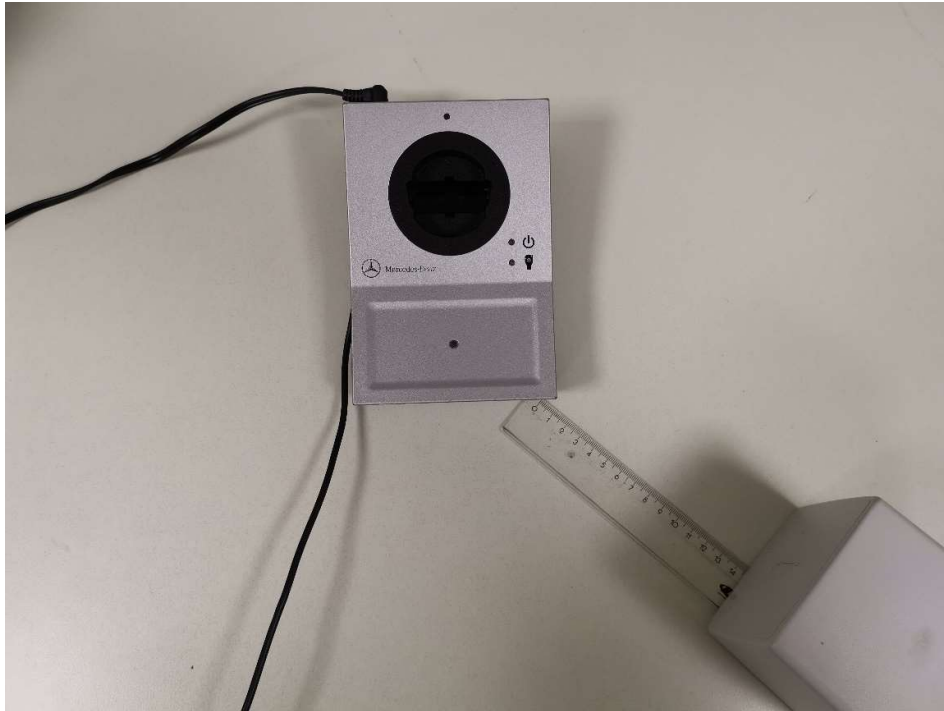
Photograph 3: Measurements in the shielded chamber, 15cm distance between measurement probe and EUT, Position 3
