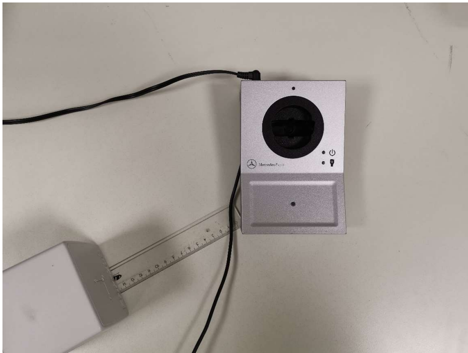
Photograph 4: Measurements in the shielded chamber, 15cm distance between measurement probe and EUT, Position 4
