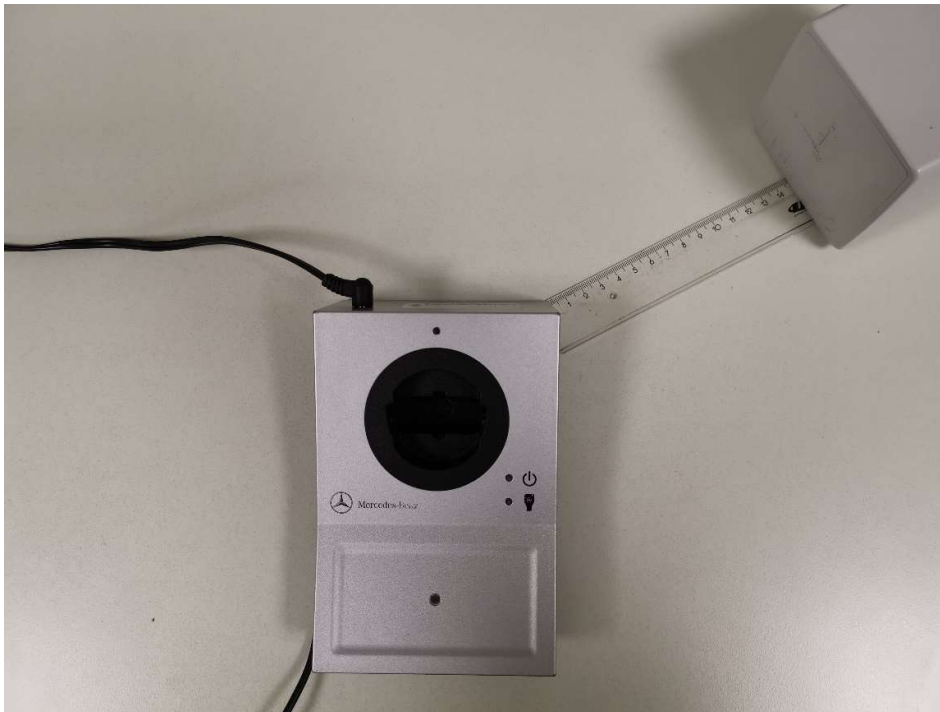
Photograph 2: Measurements in the shielded chamber, 15cm distance between measurement probe and EUT, Position 2
