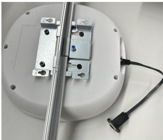
Step2. put cable into cable slot of ceiling plate
