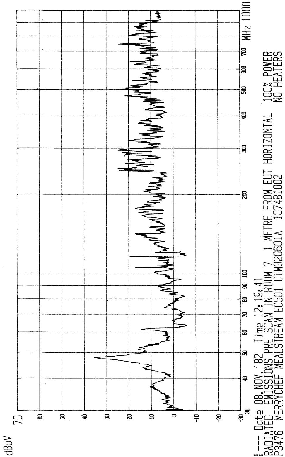
8.3.3.2 Test 3a - Figure 3 – 208V Oven – 30-1000MHz Screened Room Emission
