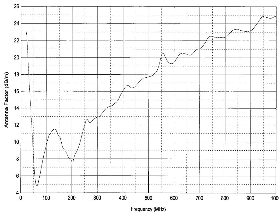
Antenna factor: Antenna model CB611A, s/n 1733.
