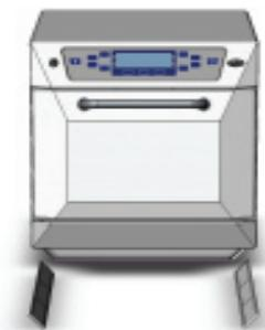
Remove the rack and lift out bottom impinger plate
