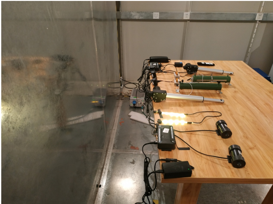
Conducted Emissions (Side View)
