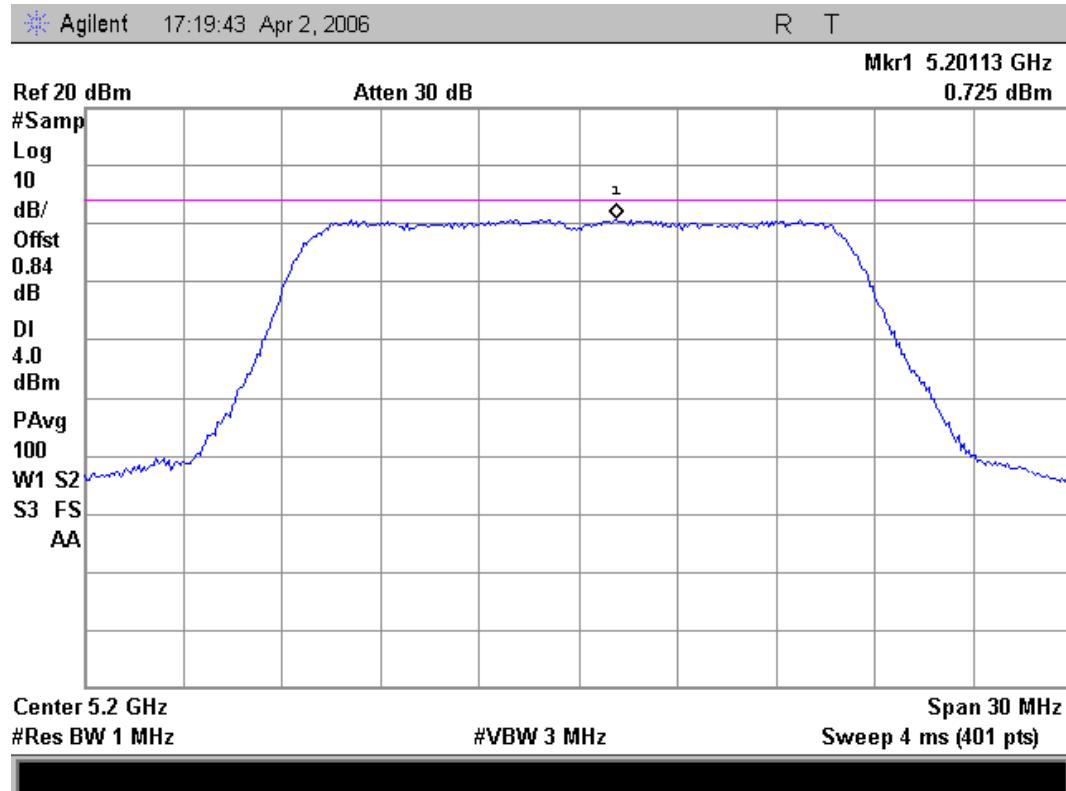
**Highest Channel (operating at 5220 MHz)**
