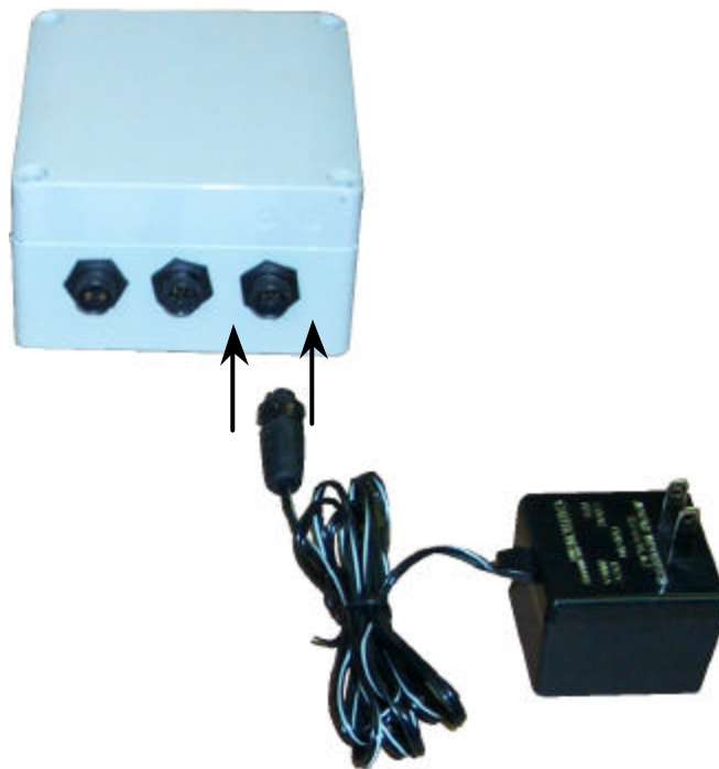
Figure 9 – 12VDC Power Supply cord hook-up
