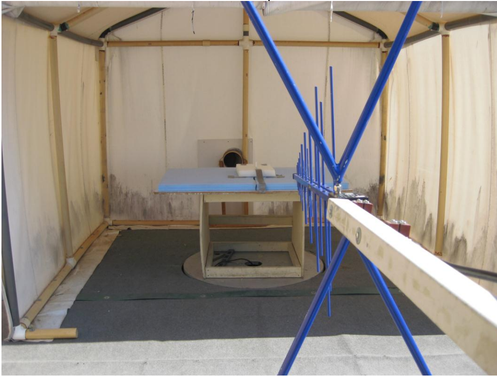
Radiated Test Set-up below 1 GHz
