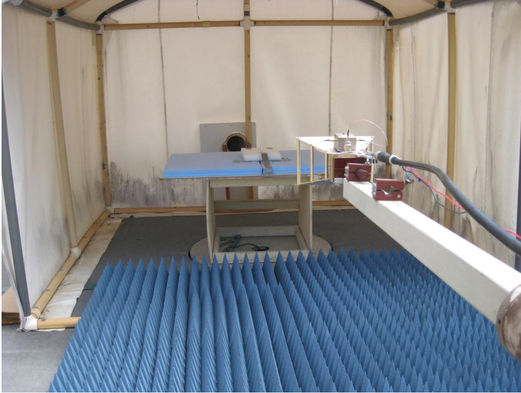
Radiated Test Set-up above 1 GHz
