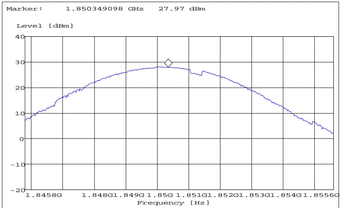
**EIRP CHANNEL 661:**
