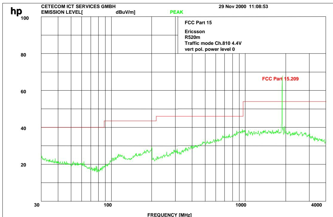
Carrier is notched with a Band Reject Filter WRCD 1879.5/1880.5-EE (Wainwright Instruments GmbH Germany)
