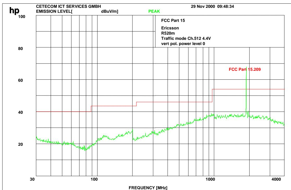
**Carrier is notched with a Band Reject Filter WRCD 1879.5/1880.5-EE (Wainwright Instruments GmbH Germany)**
