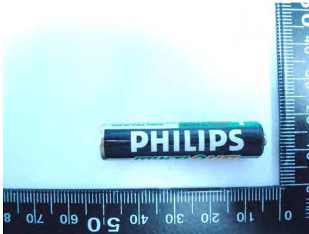
Figure 3. Battery (Ni-MH 1.2V , 750mAh)
