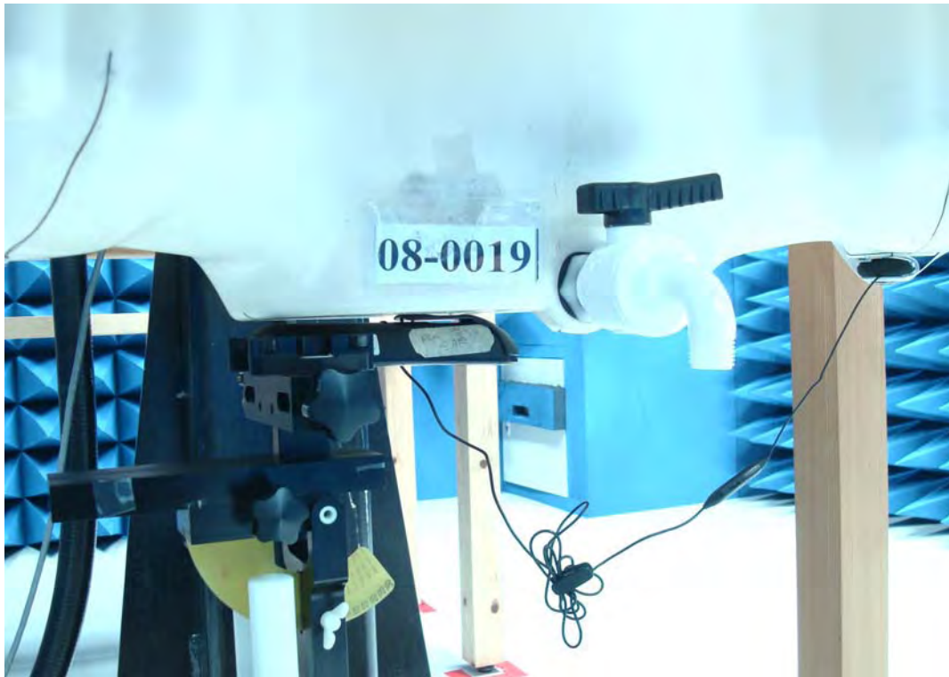
Figure 18. Body SAR Test Setup (Flat Section)
