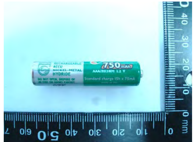
Figure 3. Battery (Ni-MH 1.2V , 750mAh)
